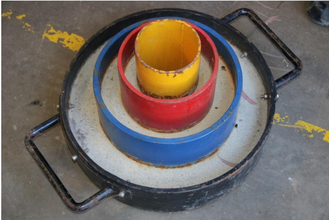
Figure 2. A display model of a triple-cased well design in cross section, viewed by the Natural Resources Committee at the Katnook Gas Plant, SA, February 2015. The centre (yellow) casing on this model is approximately 10cm across and each subsequent casing is surrounded by cement.
